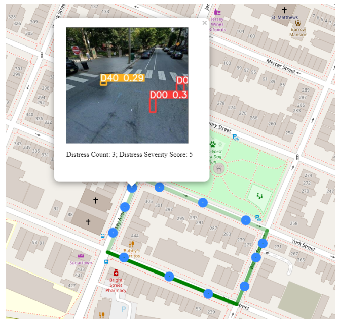
Figure 5: Folium Map of Road Distresses in Paulus Hook neighborhood in Jersey City, NJ
